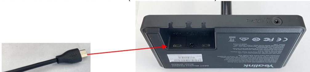
2. Connect the RJ9 end of the Headset Adapter Cable to the headset port on the side of the desk phone (Yealink T33G shown):
