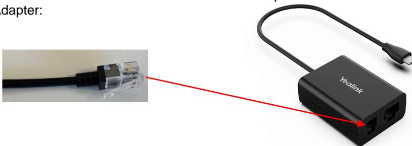
3. Connect the other RJ9 end of **Cable A** to the headset port on the back of the desk phone (VVX 450 shown):
