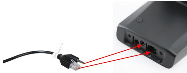
2. Plug the other two ends of the Plantronics adapter cord into the ports on the EHS40 Headset Adapter:
