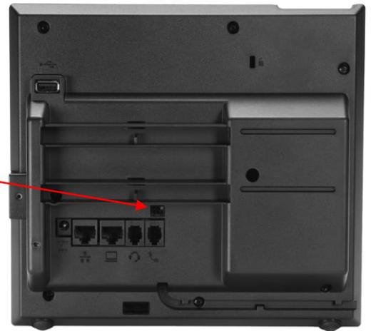
**Connect Non-Yealink Headset to Yealink T46U/T54W/T57W desk phone using EHS40 Headset Adapter Cable**
