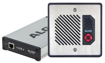
The Algo 8028 "G2" SIP Intercom is a two-component IP intercom with outdoor rated door station and separate PoE control unit. The door station requires only a single twisted pair connection allowing use of pre-existing wiring. The remotely located control unit provides connectivity to the network and door control connections eliminating any possibility of tampering for door access or network access.
