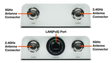
Four antenna ports on the ends of the SonicWave 231o provide connection points for the two 5GHz antennas and two 2.4GHz antennas.
