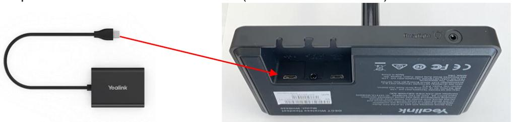
2. Connect one RJ9 end of **Cable A** to the RJ9 port on the back of the EHS60 Headset Adapter:
