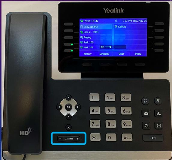
The image shows a Yealink deskphone with a color display. The screen displays a call log with the number 7632316442 and the time 1:57 PM Thu, May 05. Below the screen is a numeric keypad and a central navigation pad. A red box highlights the volume control buttons, which consist of a minus sign, a speaker icon, and a plus sign.
