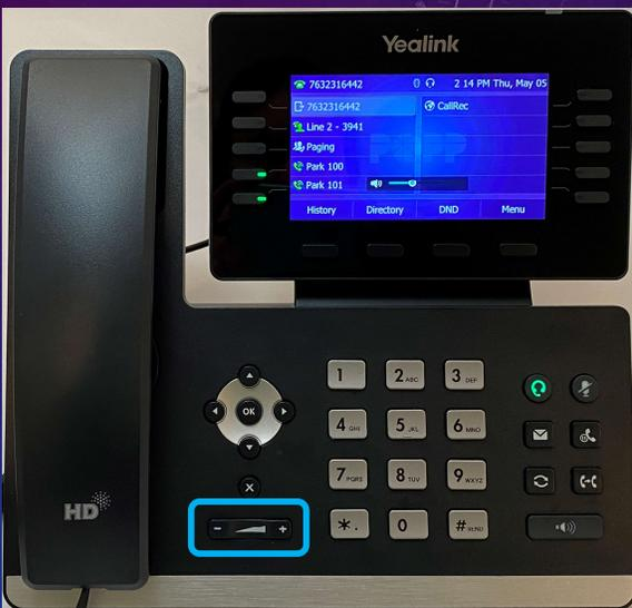
The image shows the same Yealink deskphone and headset. A blue square highlights the volume control buttons (plus and minus) located at the bottom left of the keypad.
